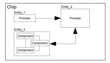
The general structure of circuits described in VHDL is composed of a heterogeneous description of dataflow and behavior between various entities and their architectures.
