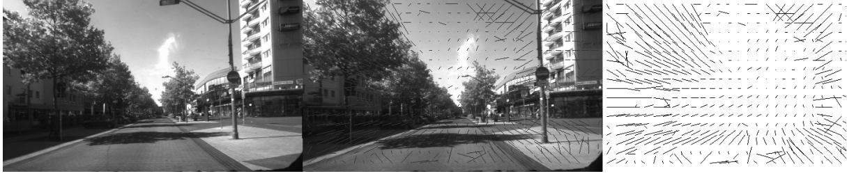
Figure 5: Resulting motion vectors, (a) first input image, (b) second image with resulting motion vector overlay, (c) vector field
